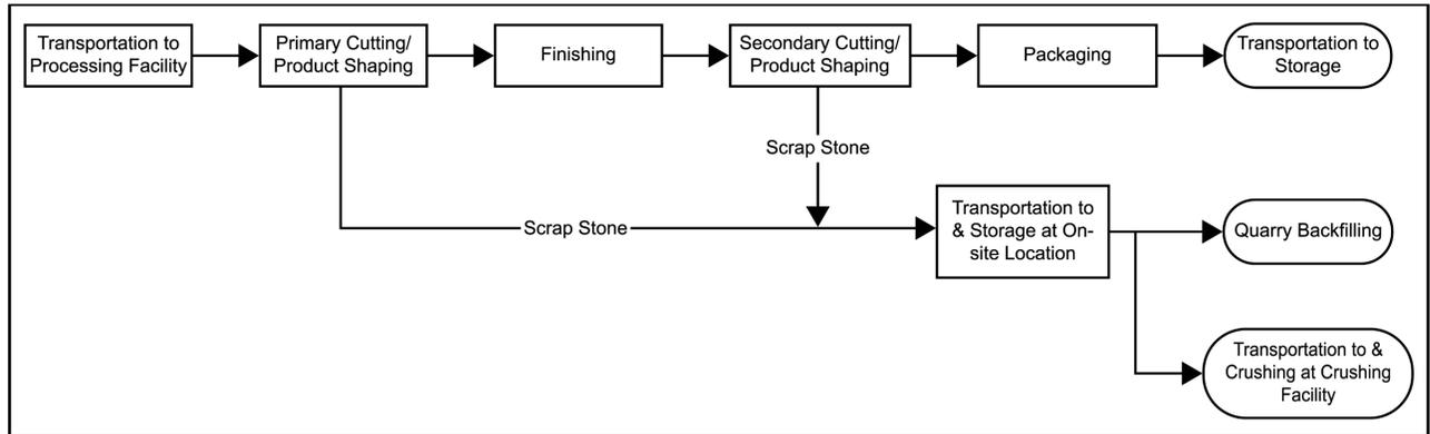
**Figure 2. Process flow diagram for granite processing operations.**
