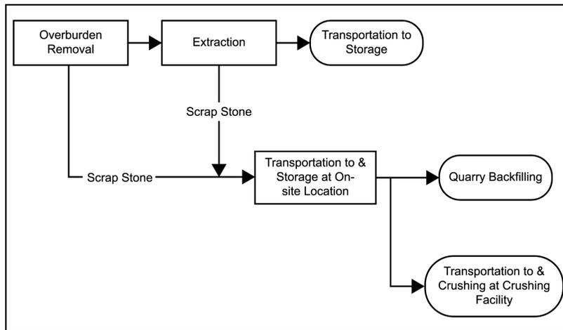
**Figure 1. Process flow diagram for granite quarrying operations.**
